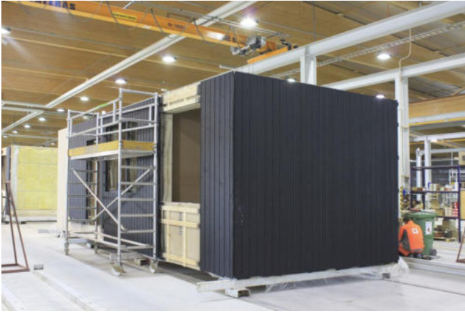
Volume elements; typical sizes: 4 500 (w) x 3 000 (h) x 13 500 (l)
